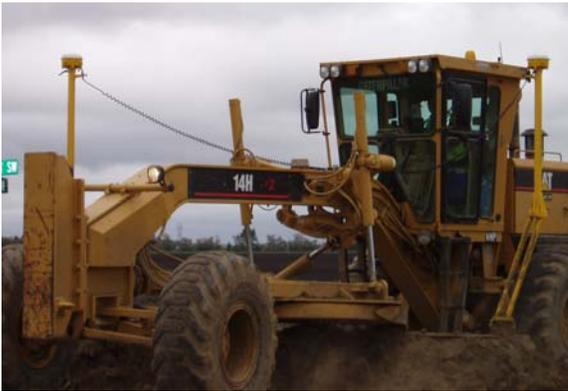
It may look like a UFO convention on the road jobs now with all the “Frisbees” sprouting off new machines, but it’s only some new GPS Machine Control. This year we felt the time was right to add to our fleet of GPS machines and we thought it would be most beneficial to expand to a scraper and a blade. One thing we noticed was that the dozers spent a lot of time telling everyone else where the grade is, and now everyone will be on the same page and we’ll be able to speed up production.
